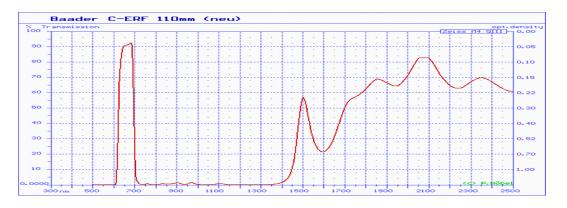
This ERF is designed for Ha observing, and provides an effective cut-off around the Ha (600nm-700nm) and above 1400nm.
